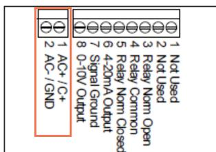
Example CO<sub>2</sub> Sensor Diagram
