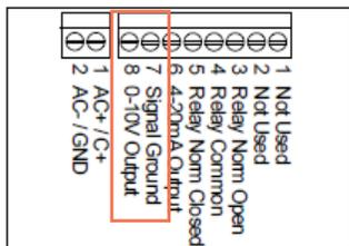
Example CO<sub>2</sub> Sensor Diagram
